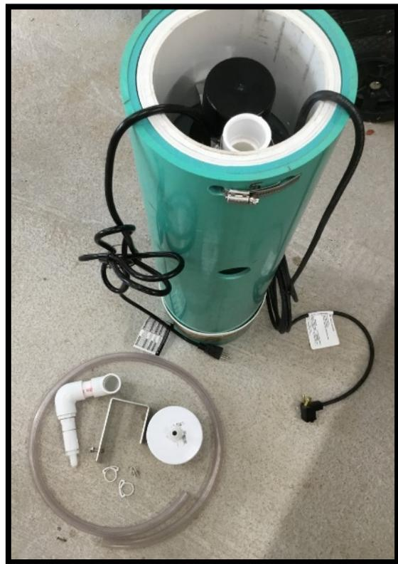
3. For installation purposes the *Septic Tank Level Control* (STLC) Filtered Pump Vault (FPV) consists of three (3) main components. The actual STLC Filter Pump Vault, the Pump Discharge Support Assembly, and the four-inch (4") Discharge Pressure Cap with barb fitting and discharge hose used to connect the FPV discharge to the septic tank outlet pipe within the septic tank.
